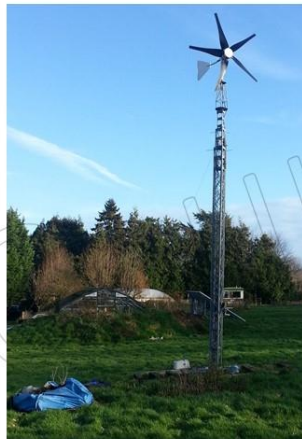
Hollow glassfibre 1kW wind turbine blades on test in Dover, UK
