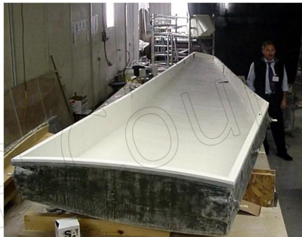
Aircraft wing Composite \frac{1}{4} scale wing for fuel flow.
