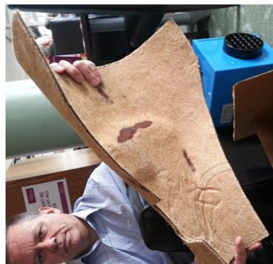
Bio Gearbox cover. Flax skin and recycled cardboard honeycomb core in BioResin
