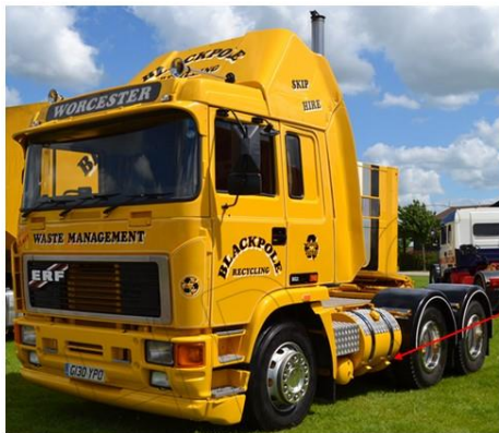
Lightweight fuel tank brackets. Final carbonfibre composite version under 2kg weight. (1995)
